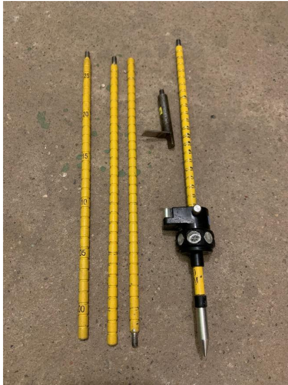
Foto 5. Miniprisma Seco Sliding 360° Prism Kit [13]
