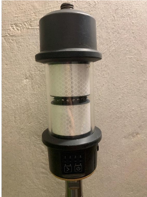
Foto 6. Põhiprisma Trimble Active Track 360° Target [13]
