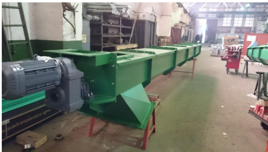
Sele 5. Kruvikonveier tootmises Ø400 L=7000 mm
