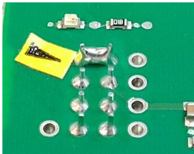
Joonis 3. Tina sild ( solder bridging ) [10]
