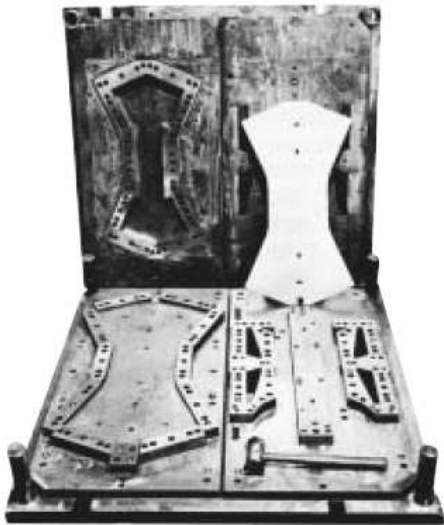
Blanking tool made from fine-machined Arne tool steel.
